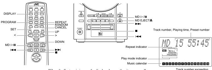
When the System is in use, the display shows other items as well. For simplicity, we show here only the items described in this section. Track number exceeding 15 is not displayed.
